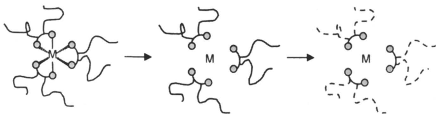
Figure 1. Schematic representation of a polymeric metal complex (left) and two stage degradation mechanism, at the metal center via macroligand dissociation (center) and along the polymer backbone (right).
